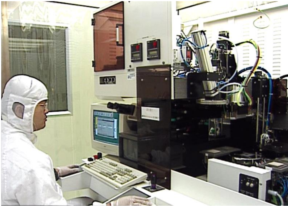
State-of-the-art Flip-Chip Bonding Equipment in 1000 m 2 (class 1000) clean room
