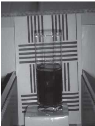
Water Absorption at Wavelength 1,300 nm (lab image) (Source: ABS GmbH, Jena)
